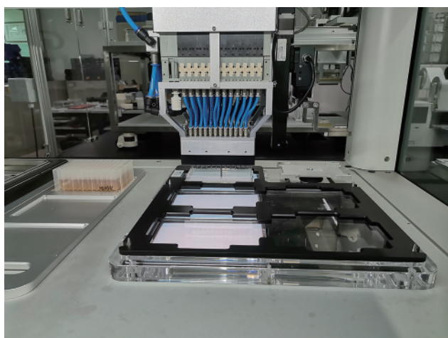
(a) 菌落图像识别挑取 (a) Colony image recognition and picking
